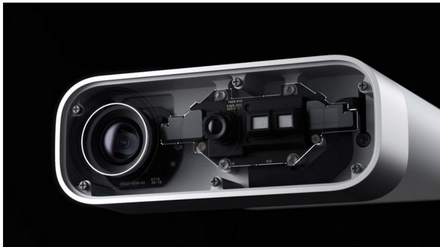
Figure 3.2: Microsoft Azure Kinect, infrared ToF camera
