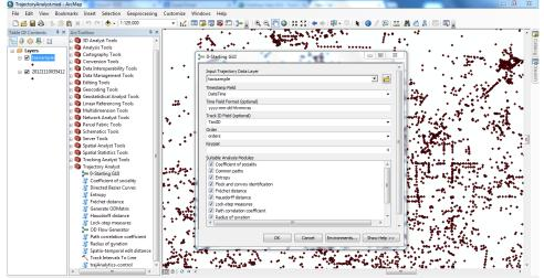
Figure 2. A screenshot of a TrajAnalyst toolbox developed in ArcGIS.
