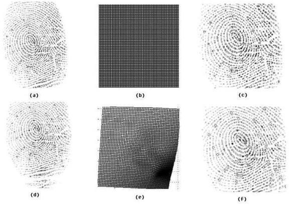
Fig. 1. TPS deformation model. (a) Template fingerprint image (b) Original Thin Plate (c) Template fingerprint image (d) Enrolled fingerprint image (e) Warped Thin Plate (f) Warped fingerprint image
