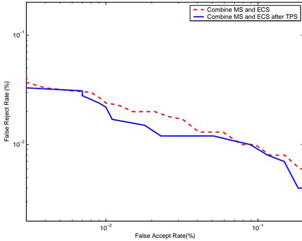
Fig. 4. ROC curves of different score combinations of DB1 data set. MS: Minutiae score. ECS: Edge correlation score. TPS: Thin-Plate Spline. Combining rule: product rule.
