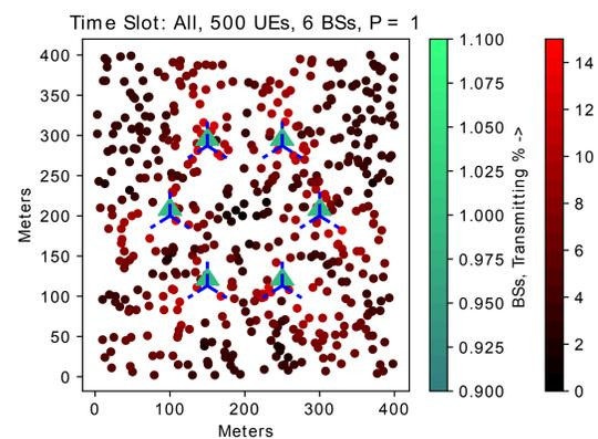
Figure: Six BSs (green triangles) with three antennas each (blue lines), and 500 UEs positioned randomly (red circles)
