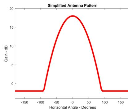
Figure: A plot of the implemented antenna pattern, with a maximum antenna gain  $G$  of 18 dB
