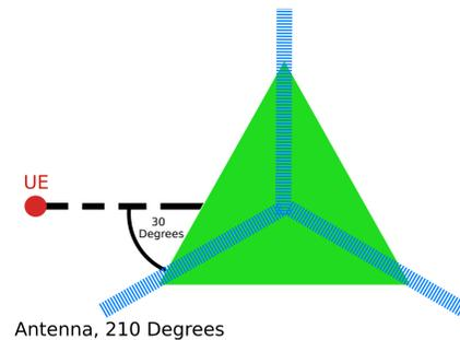
Figure: Determining the angle  $A$  between a UE and the 210 degree antenna it's associated with
