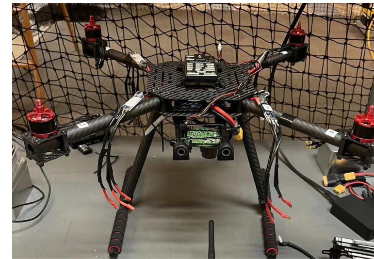
Fig. 3. IoT Drone without adding Raspberry PI 4 which can only fly with a remote controller.
