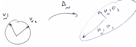
Figure 1: Transformation from hypercircle \mathbf{v} to hyperellipse \mathbf{u} with principal directions \sigma through \mathbf{A} .
