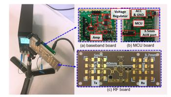
Figure 7: The implementation of 24GHz mmWave probe follows the three-board architecture: (a) a down-frequency baseband board (b) an MCU board and (c) a radio-frequency (RF) Tx/Rx board.
