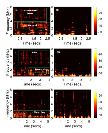
Figure 14: Spectrograms of microphone-detected signal (left) and WaveEar-sensed signal (right) with three different noises: music, presentation, and water flow. Noises cannot break into *WaveEar*.
