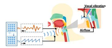
Figure 2: The vocal vibration distorts the skin-reflected mm-Wave signal. The distortion has a strong correlation with human speech.
