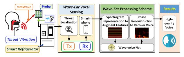
Figure 4: The system architecture for *WaveEar* mainly consisting of a mmWave sesing module in the front-end to locate and sense the vocal vibrations and Wave-voice Net in the back-end to reconstruct the high-quality voice even in the presence of ambient noise.
