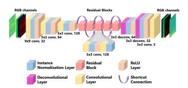
Figure 6: The structure of Wave-voice Net based on encoders and decoders to perform exhaustive extraction of speech information from voice and mmWave spectrogram.
