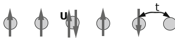
Fig. 9.1 Cartoon of the Hubbard model, characterized by a single band with near-neighbor hopping t , and local repulsion U
