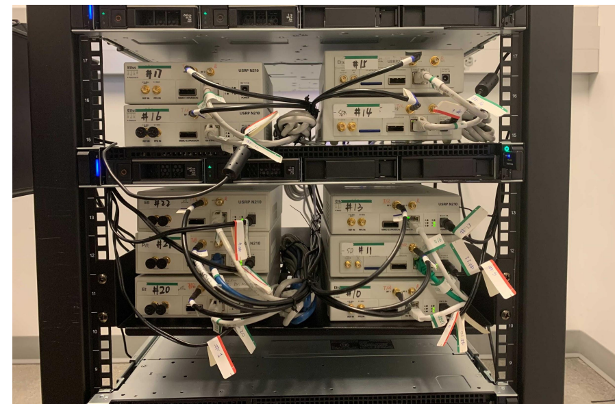
Server stack with networked USRPs
