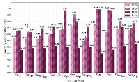
Fig. 4: PBR rate for QPSK-modulated data streams with packet size of 1500, 2000, 4000 bytes and random size.
