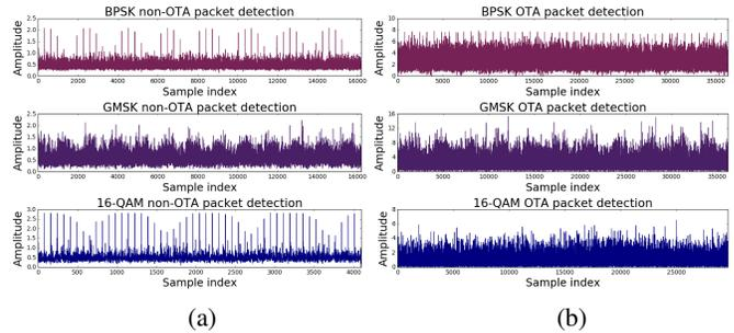
Fig. 3: Example PBR output using sensed signals (Welch's method). (a) Example of non-OTA data; (b) Example of sensed OTA data.
