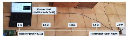
Fig. 2: A snapshot of the software-defined PBR testbed.
