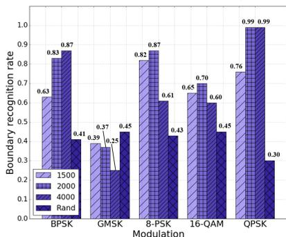
Fig. 5: Analysis of modulation for KLD, 2000-byte packets.
