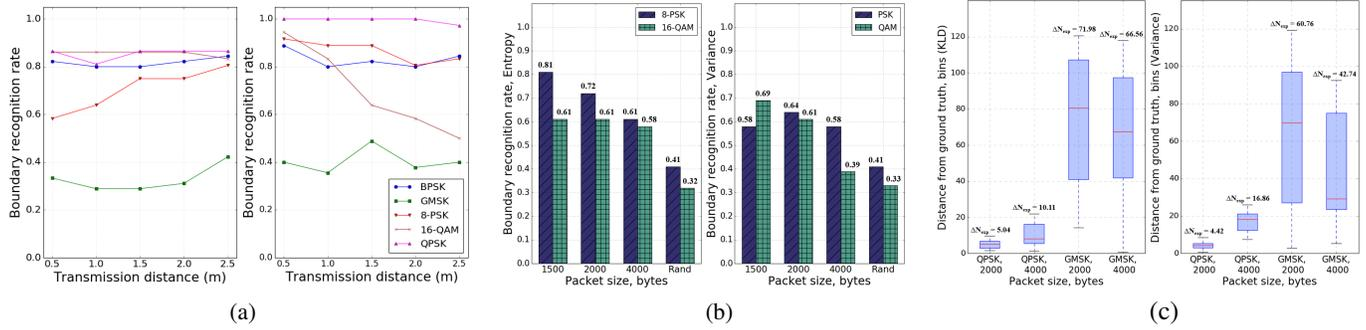
Fig. 6: Performance metrics of various test configurations. (a) PBR rate against transmission distance with bin size of 50 (left) and 100 (right) samples; (b) PBR rates with different packet sizes for entropy (left) and variance (right) approaches; and (c) PBR accuracy of KLD (left) and variance (right) approaches.
