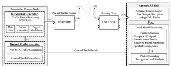
Fig. 1: Software-defined packet recognition framework.
