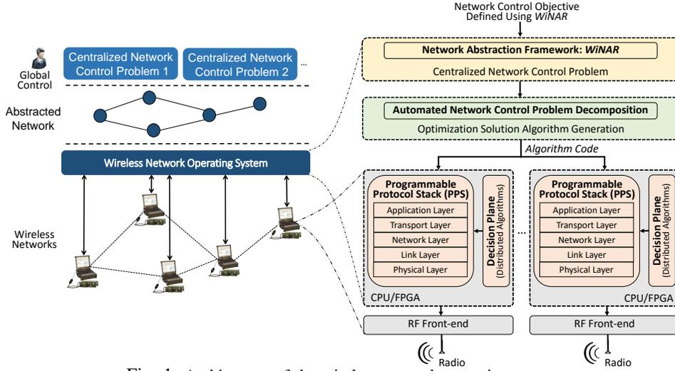
Fig. 1: Architecture of the wireless network operating system.
