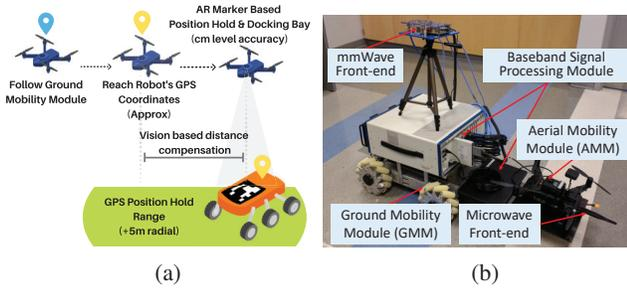
Fig. 3. (a) Synchronization of the aerial and ground mobility modules; (b) Prototype of UBSpot.
