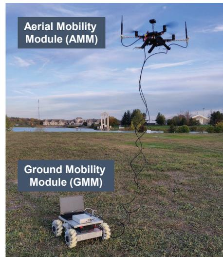
Fig. 4. Experimental setup for synchronized movement of aerial and ground mobility modules.
