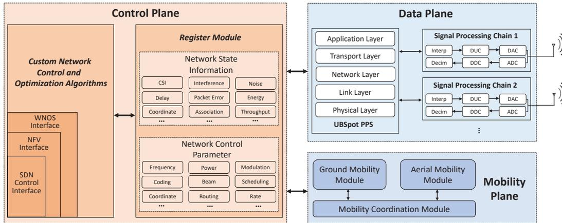
Fig. 2. Architecture of UBSpot: A universal broadband flying hotspot for software-defined aerial-ground wireless networking.
