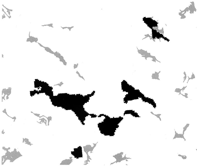
Figure 1. Flat objects used to guide search for flow paths. Dark objects are classified as water bodies.
