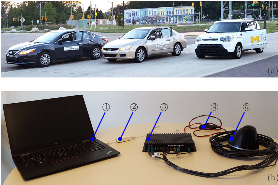
Fig. 4. (a) Two human-driven vehicles and one connected automated vehicle used in the experiments. The two vehicles on the left are only equipped with V2X communication devices, while the vehicle on the right is capable of automated driving as well as V2X communication. (b) The V2X communication device: 1 upper-level computer, 2 ethernet cable, 3 electronic control unit, 4 power cable, 5 GPS and V2X antennae.
