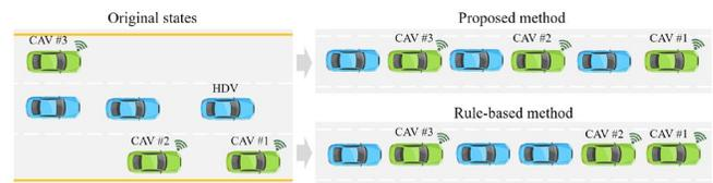
Fig. 12. The formed mixed vehicle platoon using rule-based and proposed methods.
