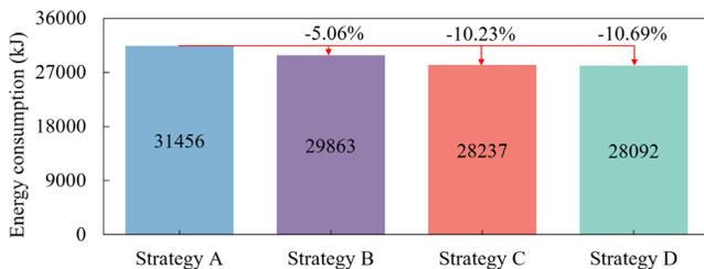
Fig. 16. The average energy of mixed vehicle platoon in whole travel.
