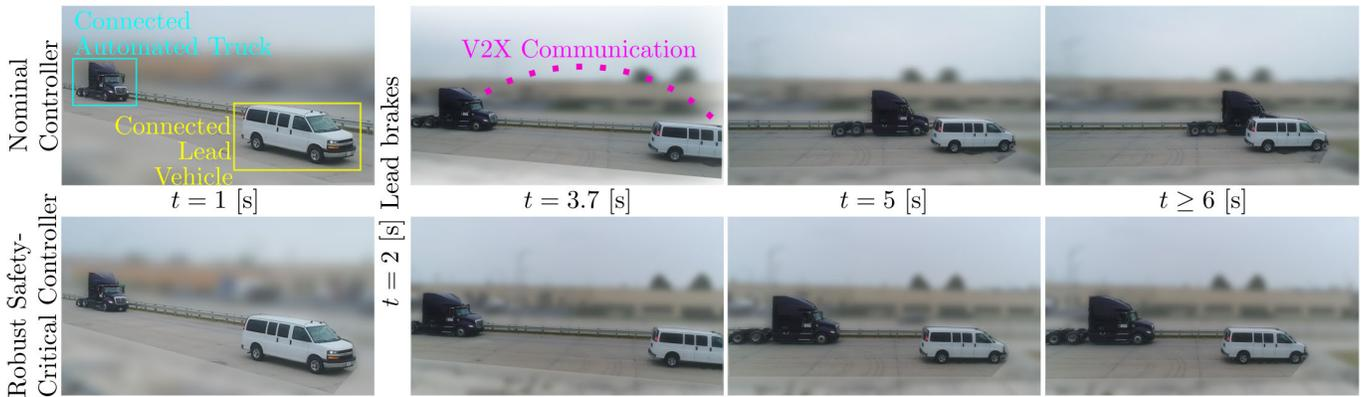
Fig. 1. Experimental configuration for heavy-duty CAV problem. (Top) Controller design without robustifying element yields safety violation. (Bottom) Robust safety-critical controller ensures CAV brakes early and aggressively enough to maintain safe distance.
