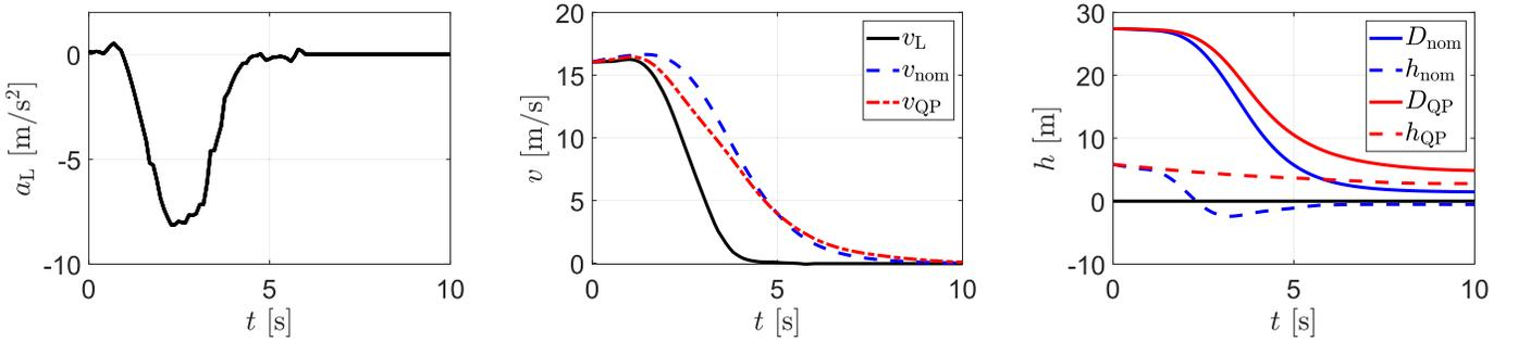
Fig. 12. (Left) Example profile for acceleration  $a_L$  of lead vehicle used in numerical simulation. (Center) Velocity  $v_L$  of lead vehicle (black) and velocity of the truck using the nominal controller (53) (blue) and safety-critical controller (57) (red). (Right) Following distance  $D$  and value of CBF  $h$  using the nominal controller and safety-critical controller.
