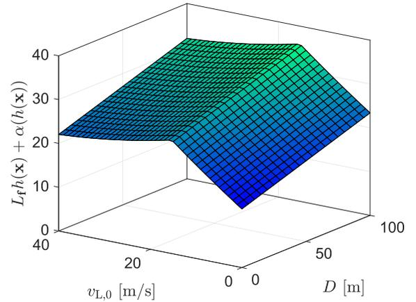
Fig. 10. Value of  $L_f h(\mathbf{x}) + \alpha(h(\mathbf{x}))$  as defined in (52) when  $L_g h(\mathbf{x}) = 0$  for various distances. As the function is strictly positive over the domain of interest,  $h$  is a CBF on  $\mathcal{C}$  for (46).
