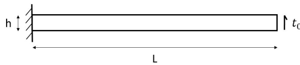
Figure 4: Schematic of a cantilever beam
