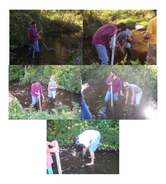
In the last part, the velocity was found using the Marsh-McBirney Flo-Mate model 2000 electromagnetic current meter. The same steps were repeated as the previous section of the lab.
