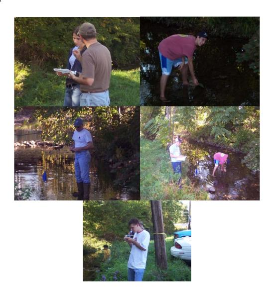
In the next part of the lab a positions was selected, and the channel width (wi), and the flow depth (di) recorded. Using the price current meter #625 the number of licks (turns of the wheel) were recorded for 60-120 sec intervals to determine the velocity of the water. This was done a few times going across the channel.
