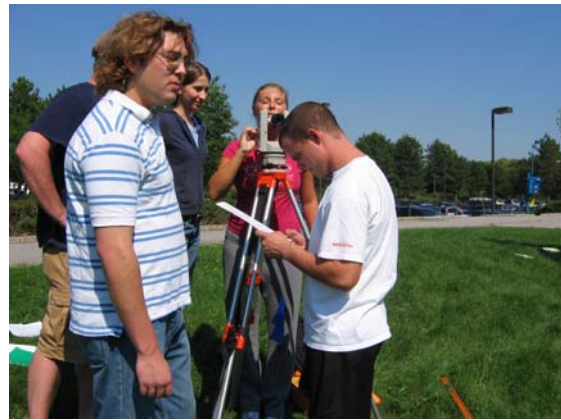
Secondly, level the theodolite's base and its telescope.
