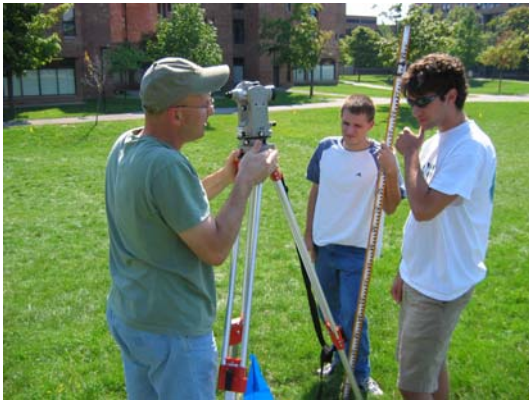
First setup the tripod steadily and level; and then place theodolite onto it, securely.
