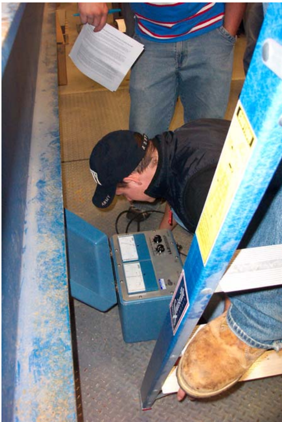
Here is a group trying to accurately read the bouncing dial of the Model 523
