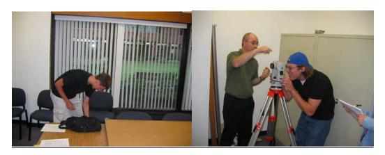
Using blocks we changed the elevation and using the Theodolite we determined the relative elevation using up to three blocks.
