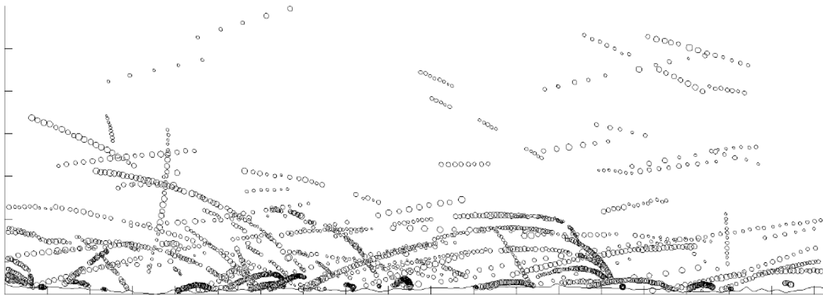
Figure 1. Sample of 250 sand particle trajectory segments captured in 0.25 s using the EPAS PTV system. Freestream velocity was 8 \text{ ms}^{-1} . Interval between tick marks is 5 mm.
