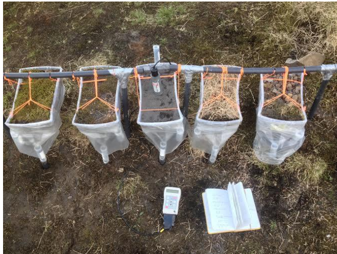
Figure 1. Experimental field set-up of infiltration experiment, June, 2015. Each plot is 537 cm 2 and infiltrating water can be stored in the soil matrix, runoff or freely drain into a measuring vessel. Surficial materials are typical of the study slope. Left to right is: Moss, Ash Blasted Moss, Grass (no Ash), and a mix of Rock, Grass+Ash blasted Moss. The set-up can adjust for aspect and slope angle. Note a Theta soil moisture meter monitors volumetric soil moisture in the Ash plot.
