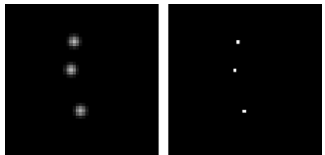
Fig. 7. Demonstration of simple thresholding technique. (left) Single frame slit image before thresholding. (right) Image after thresholding.
