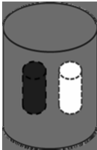
Figure 4. A diagram illustrating the composition of the contrast phantom. The small black and white cylinders were filled with ^{99m}\text{Tc} solution and water, respectively. The main cylinder was filled with background activity.
