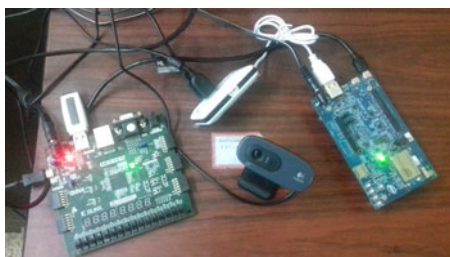
Fig. 7. Experimental setup for smart IoT node.
