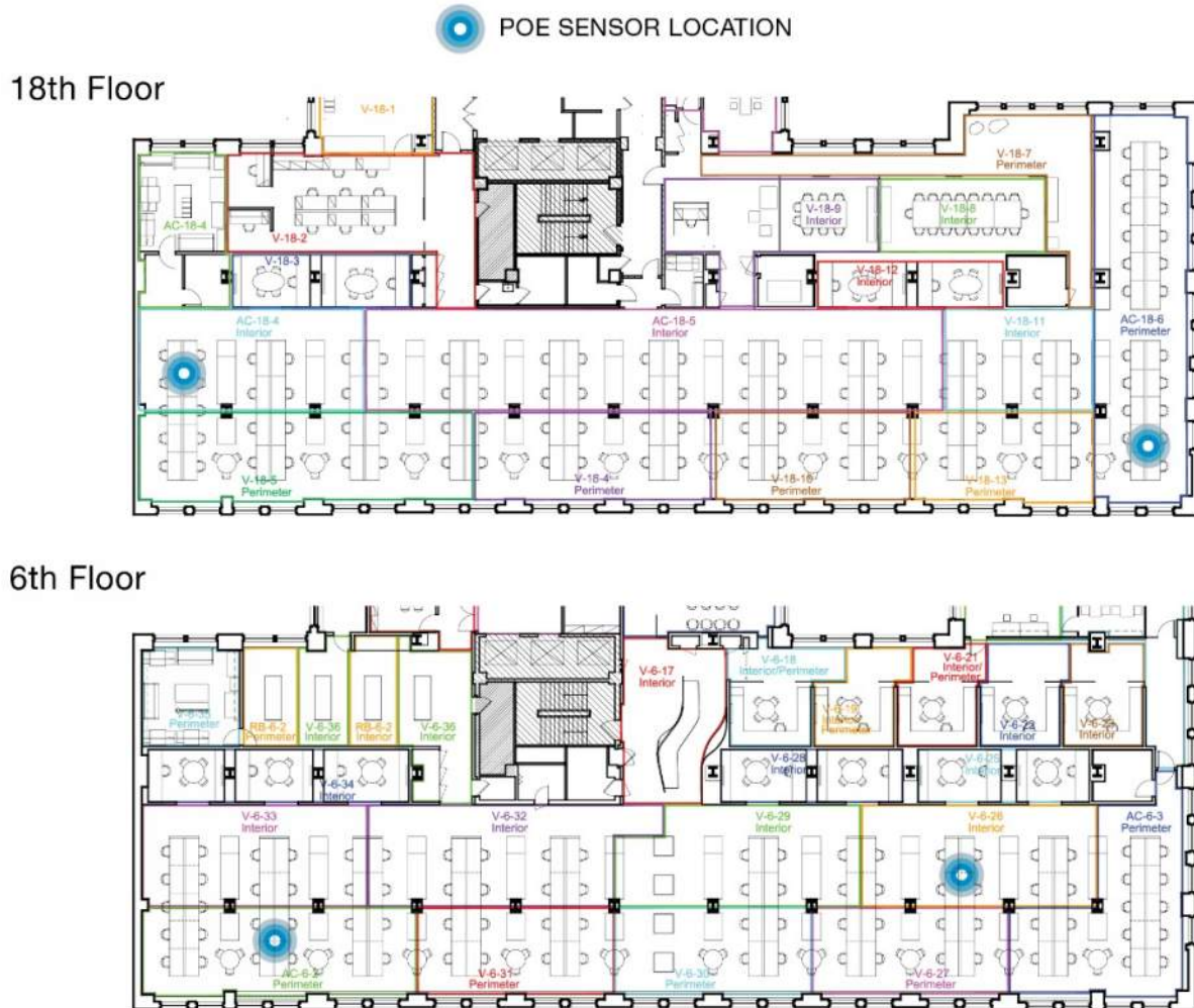
Figure 2: Office POE sensor locations, also showing building mechanical zones
