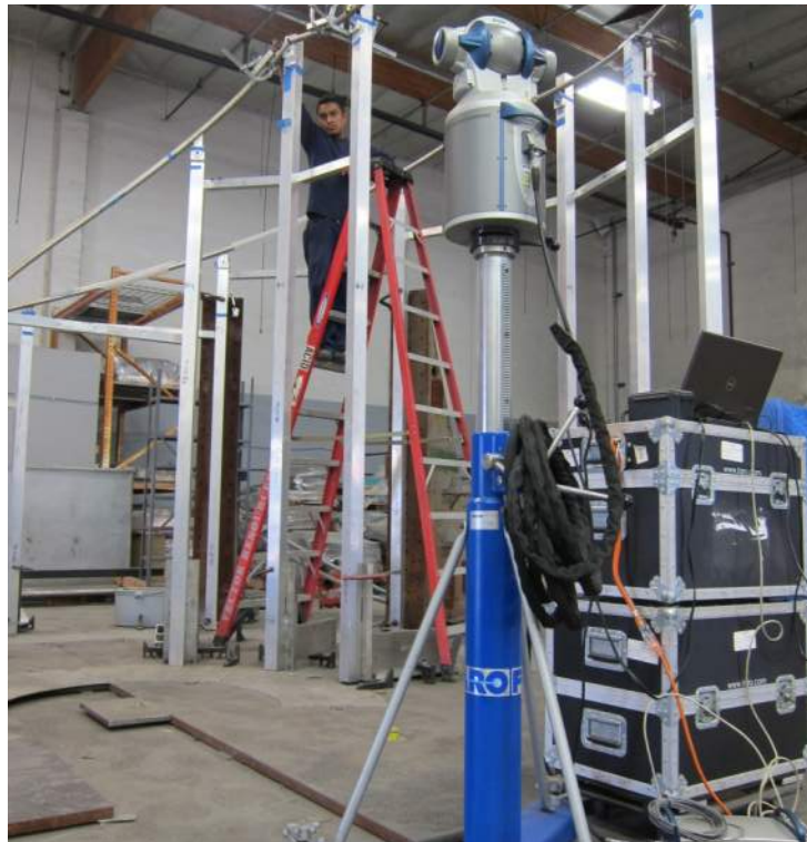
Figure 13: The head of this laser tracker follows the target (held by the operator) as the target is moved through 3D space. The operator can read the location of the target's center directly off the laptop's screen. (photo by the author)
