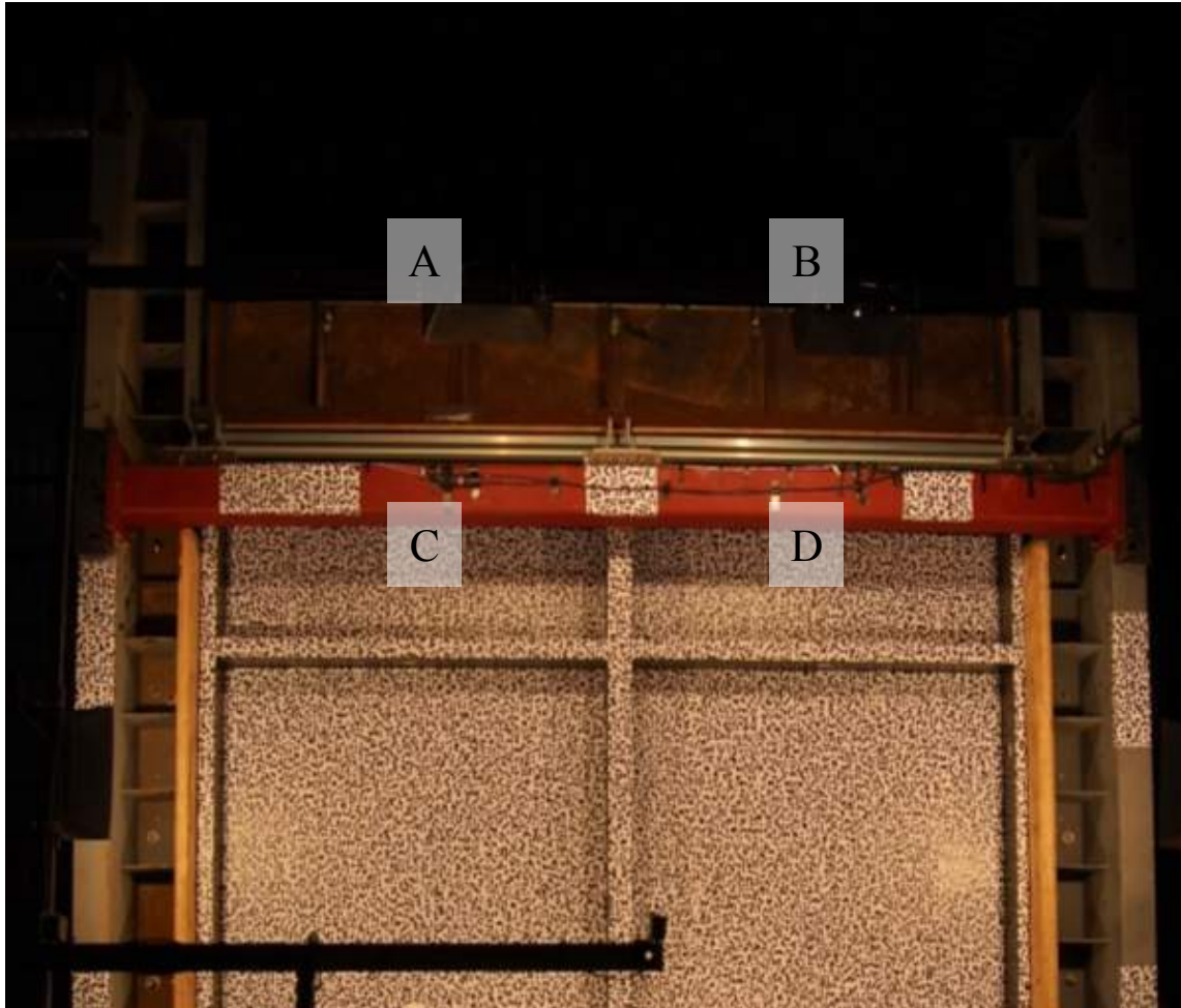
Figure 6. DIC Speckle Pattern
