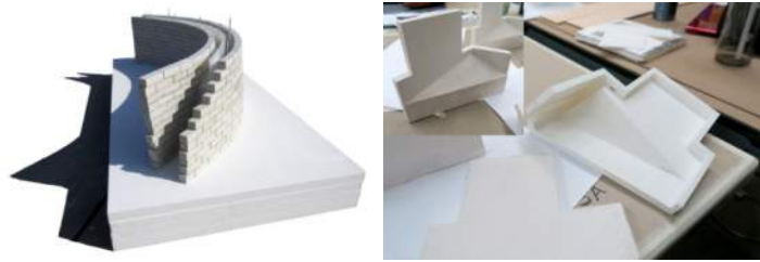
Figure 7: A model of a section of the brick construction of Frank Lloyd Wright's Johnson Wax Building by Yukie Takeshi and Amanda Woo made from molds that were laser cut . Figure 8: 3d printed molds and plaster wall models of James Stirling's Andrew Melville Hall made by Necils Lopez, Yanelli Monjaras, and Pedro Cuin-Molinero, Pedro.
