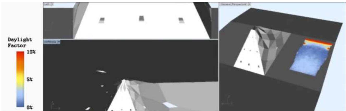
Figure 13: A combination of a small skylight and a high granularity for the façade, with a large number of punctures holes, created an over lit environment for the spa.
