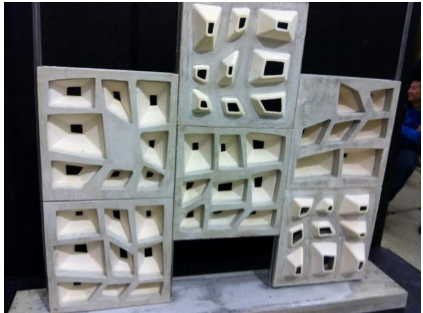
Figure 1: The geometry of the pine cone surface (left) served as inspiration to the building skin concept developed by student Eleftheria Stavridi in the first semester of Studio One (right). The physical mockup was built out of concrete, with white ceramic inserts.
