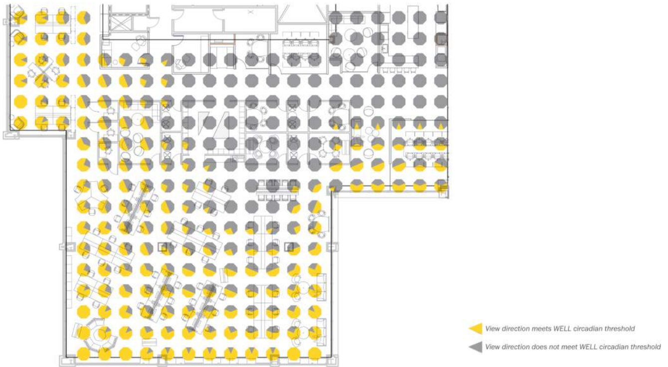
Figure 3: Method 2 circadian daylight results. A point with a view facing any of the yellow orientations in a given location meets the WELL circadian threshold (image courtesy of Atelier Ten).
