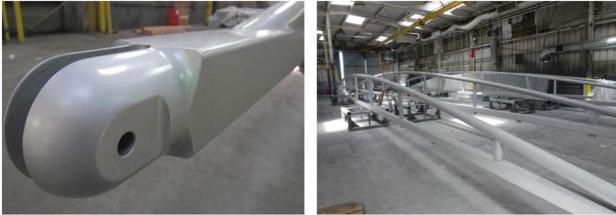
Figure 31. The precision of the steel trusses at 601 Mass Ave in Washington provided both the dimensional accuracy needed to properly capture the glass lites and a level of fit and finish that is not otherwise achievable. In 4 of the 18 building connection locations custom mounting brackets had to be fashioned to accommodate steel outside of the agreed upon tolerance band. (photo by the author)
