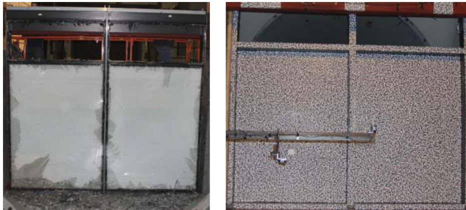
Figure 14. Test 4 Blast Side (left) and Protected Side (right)
