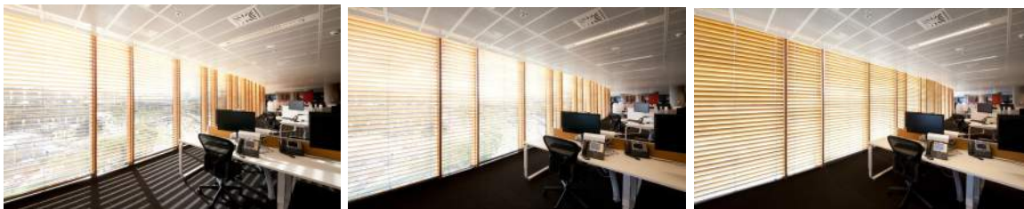
Figure 2: Darling Walk in Sydney with the blinds in three separate degrees of closing, note the nature of the lighting caused by the properties of the timber blind.
