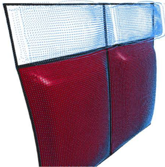
Figure 13. FEA Representation of Glass-Break Methodology in LS-DYNA
