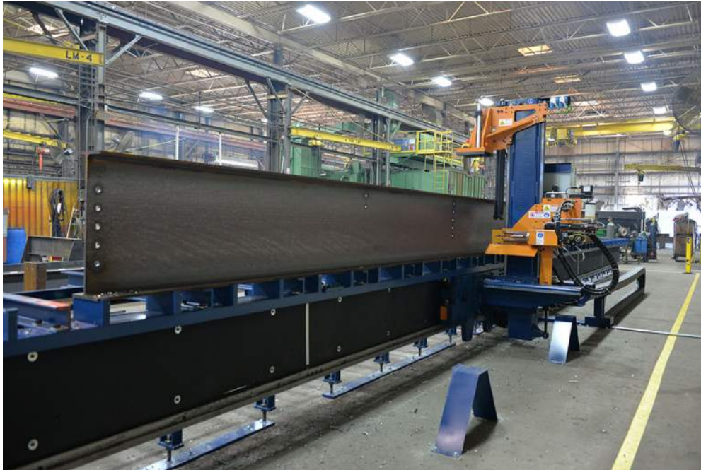
Figure 10: A CNC beam line for the automated cutting and drilling of structural steel. (photo courtesy of TMG Machine)
