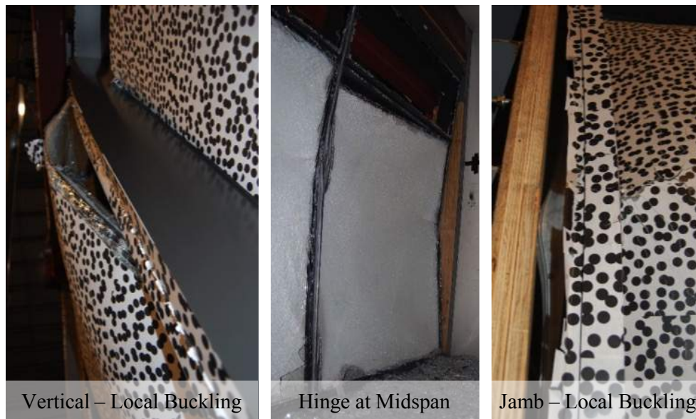
Figure 10. Vertical Mullion and Jamb Response – Test 5
