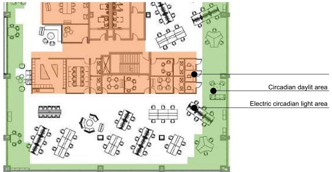
Figure 5: Zones defining the proposed integrated daylight and circadian electric light approach (courtesy of Atelier Ten)
