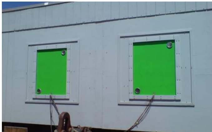
Figure 2: Medium-scale experimental and control units installed in calorimetric chambers. Image courtesy of Architectural Applications.
