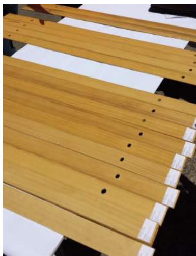
Figure 4: Indicates sampling for color variation range for blind slats on 200 George Street Sydney project
