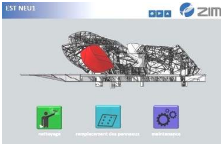
Figure 12: Screenshot of the access and maintenance management system (image by the author)
