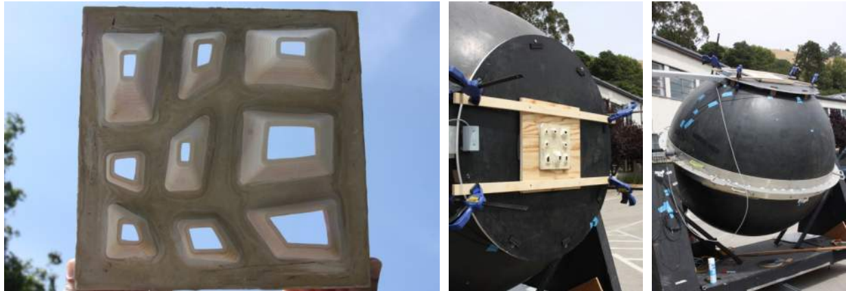
Figure 7: Left: 20x20 cm physical prototype used for light transmission measurements. Middle: View of sample attached to the Integrating Sphere at Lawrence Berkeley National Laboratory, in the 'outside facing' position. Right: View of Integrating Sphere while rotating for measurement of light transmission at different incident angles.
