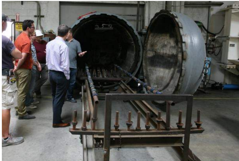
Figures 4 and 5: These images show part of the process to insert the PVB interlayer between the slumped glass panes developed for The Gores Group Headquarters – left shows the slumped glass panels with PVB interlayer prior to being vacuum sealed (the pattern only appears after the sealing process); right, the design team is being shown the autoclave where the final vacuum-sealing of the panels is done. (Photo credit withheld to maintain anonymity during review)
