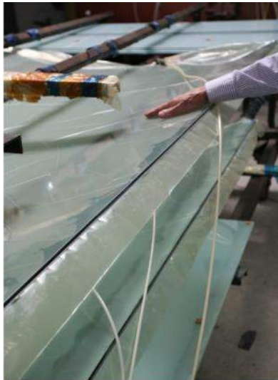
Figures 4 and 5: These images show part of the process to insert the PVB interlayer between the slumped glass panes developed for The Gores Group Headquarters – left shows the slumped glass panels with PVB interlayer prior to being vacuum sealed (the pattern only appears after the sealing process); right, the design team is being shown the autoclave where the final vacuum-sealing of the panels is done. (Photo credit withheld to maintain anonymity during review)
