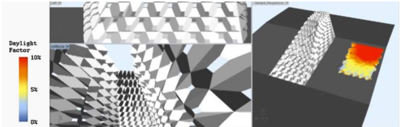
Figure 14: A combination of a large skylight and a high granularity for the façade, with a large number of punctures holes, created an over lit environment for the spa. The off-centered skylight promotes an uneven pattern of light.
