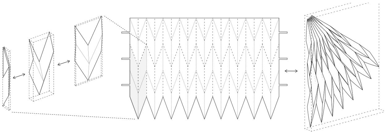
△ Figure 8. Diagram of a folding mechanism.
