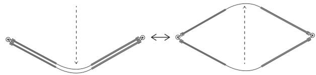
△ Figure 1. Open and closed diagrams using snapping beams.
