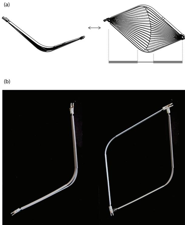
△ Figure 5. Base module of the snap deformation: (a) drawing; (b) developed prototype structure.
