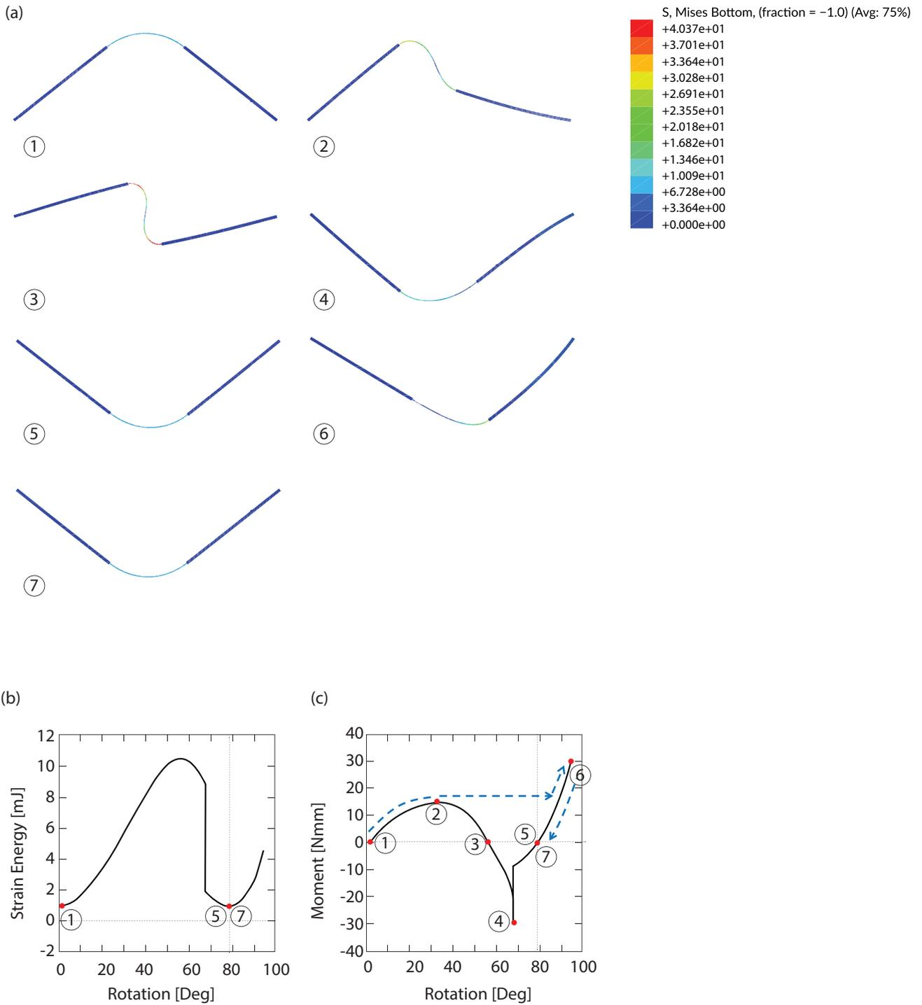
△ Figure 4. (a) progressive deformed shapes of the FE analysis; (b) relationship between rotation angle and the corresponding strain energy stored in the structure; (c) relationship between rotation angle and the applied moment.
