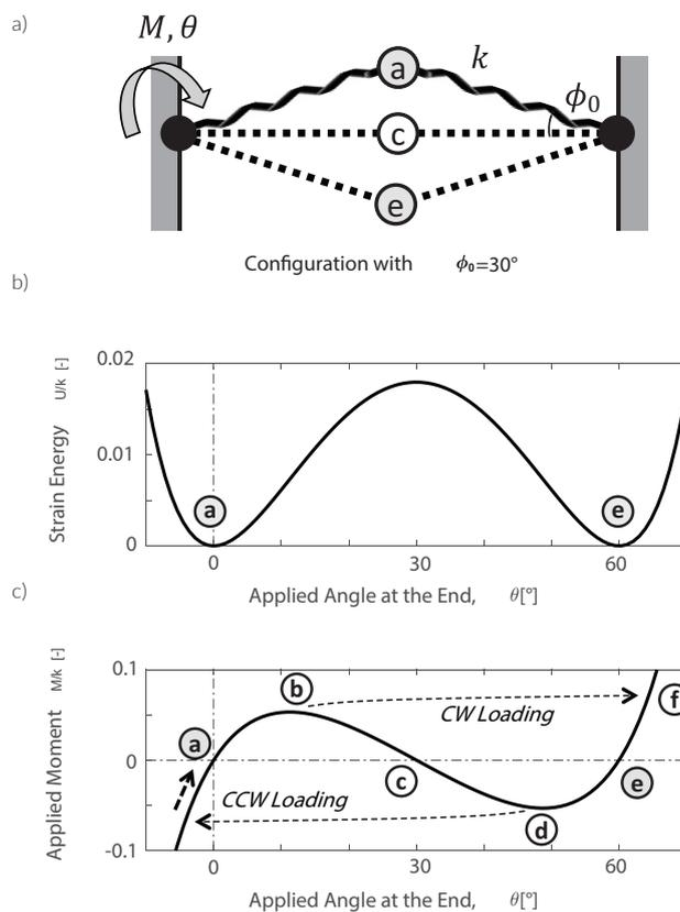
△ Figure 3. (a) Schematic of a simple bistable structure. (b) Relationship between the rotation angle and the corresponding strain energy stored in the structure. (c) Relationship between the rotation angle and the applied moment.
