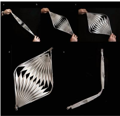
△ Figure 9. Membrane in a snapping facade base module.
