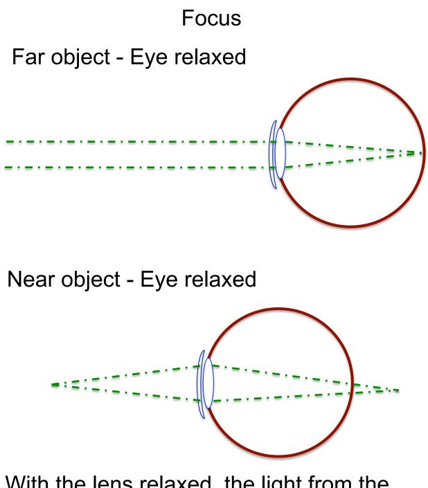
With the lens relaxed, the light from the object is not bent enough to focus on the retina
