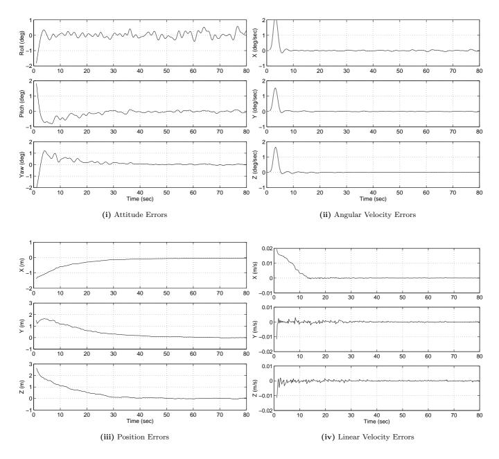
Figure 7: Attitude and Angular Velocity Errors, and Position and Linear Velocity Errors
