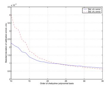
Figure 4: Order of Polynomials Versus Calibration Accuracy
