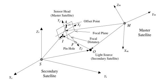
Figure 1: Focal Plane Measurement from One Light Source
