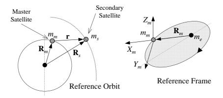
Figure 5: Relative Navigation: Master and Secondary Satellite Orbits
