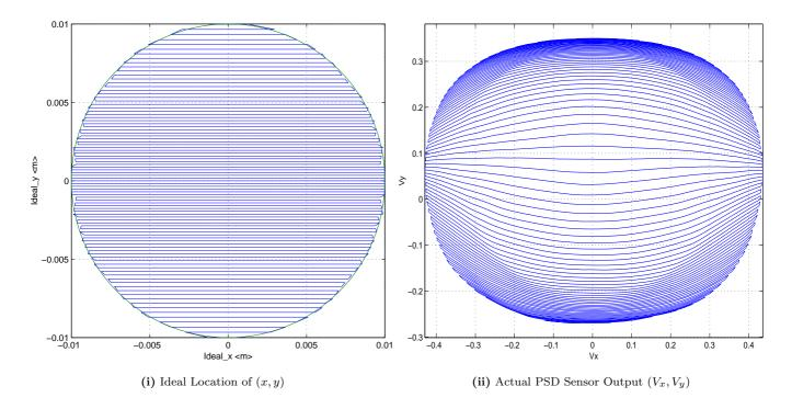
Figure 2: Ideal Location and Actual PSD Sensor Output
