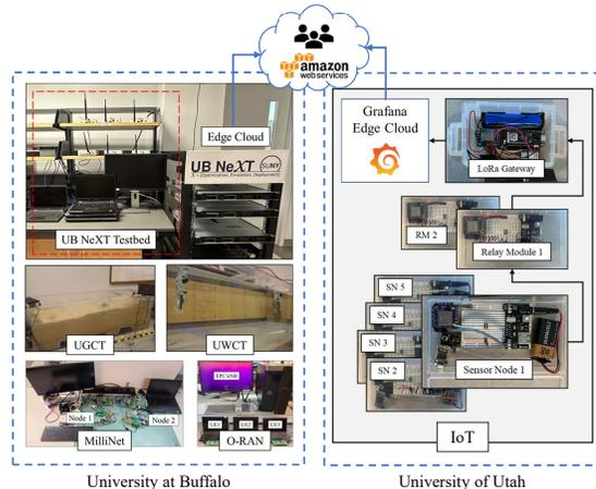
Fig. 2: Federated testbeds (from top left): UB NeXT, UGCT, UWCT, MilliNet, O-RAN, and IoT Testbed.
