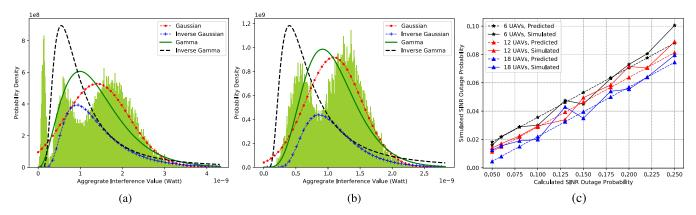
Fig. 5. Aggregate interference pdf with (a) 10 and (b) 20 UAVs; (c) Validation of data-driven prediction of the SINR outage probability for the incumbent system.
