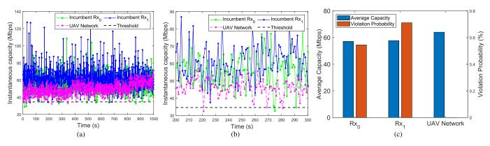
Fig. 15. Spectrum sharing between two incumbent user pairs and 6 UAVs. (a) Instantaneous capacity of the incumbent system and the UAV network; (b) zoomed in plot of time slots 200-300; and (c) average capacity and violation probability.
