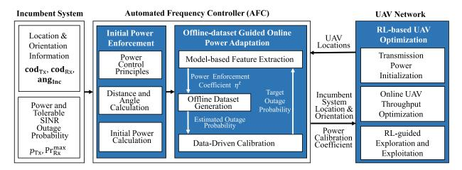
Fig. 2. Diagram of the SwarmShare spectrum sharing framework.
