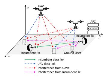
Fig. 1. Spectrum sharing between coexisting UAV network and the incumbent network in the 6 GHz bands.
