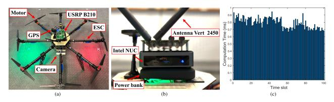
Fig. 14. (a) Snapshot of octocopter UAV, (b) onboard computing device Intel NUC, and (c) computation time.
