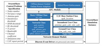
Fig. 4. Diagram of UBSim-based SwarmShare simulator.
