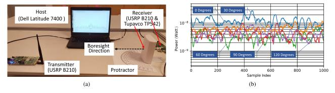
Fig. 3. (a) Snapshot of the testbed setup for threshold angle measurement; (b) Examples of the measurement results.
