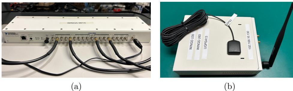
Figure 4.14: (a) Snapshot of the Octoclock; (b) GPS module
