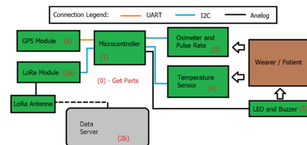
Data collection for the device is based upon the use of I<sup>2</sup>C and UART communication channels, with the microcontroller firmware collecting periodic data from the MAX30102, MLX90614, and GT-U7 components. Simple processing algorithms trigger an alert when the values are outside of a preset range. If an alert is triggered, the device will provide the type of alert and GPS data for the location to the LoRa gateway.
