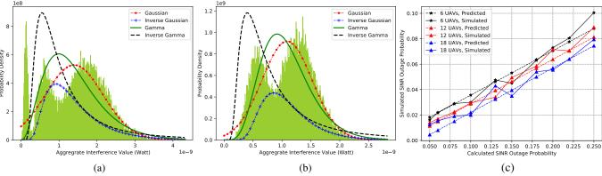
Fig. 3: Aggregate interference pdf with (a) 10 and (b) 20 UAVs; (c) Validation of data-driven predication of the SINR outage probability for the incumbent system.
