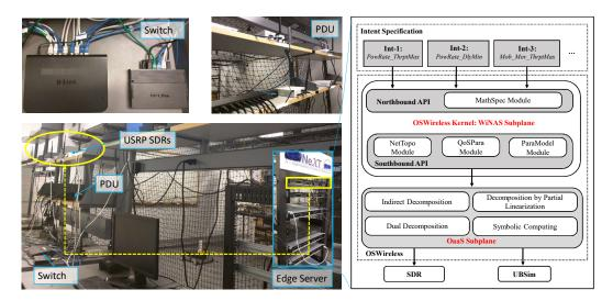
Figure 6: Snapshot of the software-defined testbed and software diagram for OSWireless prototyping.
