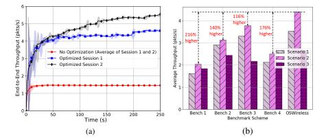
Figure 9: (a) Single-run running average and (b) multi-run average end-to-end throughput achieved by OSWireless generated control programs for MSMH\_PowRate\_ThrptMax.
