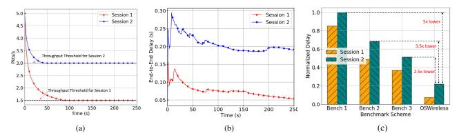
Figure 11: Instantaneous (a) transmission rate and (b) end-to-end delay; (c) average end-to-end delay.
