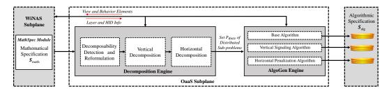
Figure 5: Overall architecture of Optimization-as-a-Service (OaaS) Subplane.
