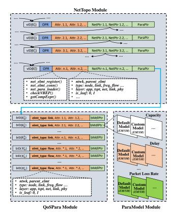
Figure 3: Diagram of NetTopo, QoSPara and ParaModel modules. These three modules together provide various kernel services for the other modules of OSWireless.
