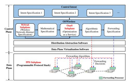
Figure 1: Overall architecture of OSWireless.
