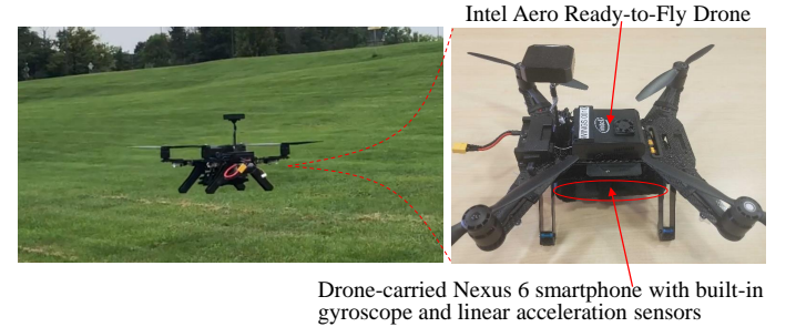
Fig. 3: Field measurement of drone flight uncertainties.
