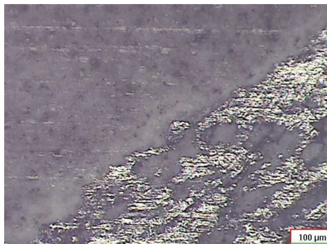
Fig. 2—Optical microscope photograph of polished surface of cement paste containing untreated silica fume and graphite network cementitious admixture. Part of edge of piece of this admixture is shown at right lower portion of photo. Bright regions are graphite, which has probably been smeared by polishing, as suggested by slightly shiny appearance of admixture edge. Dark regions are cement.
