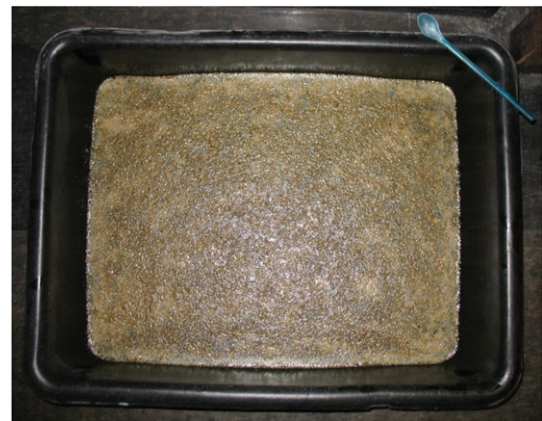
Fig. 2. Coagulation of oil in water, using bentonite, sawdust and calcium hydroxide (formulation (ii)) in medium-scale testing. Top view of the container, showing the coagulated material in a sheet form floating on the water in the container. The spoon used in this paper is also shown.
