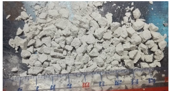
Fig. 2 Gypsum particles used as an admixture to provide defective cement paste. The scale nearest the gypsum particles has the smallest division in mm
