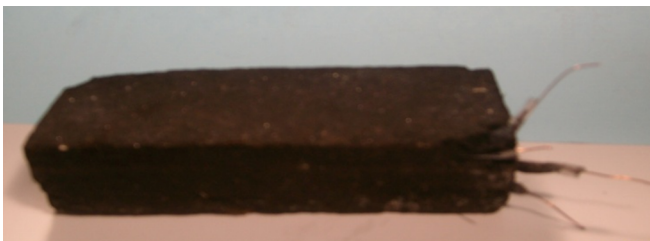
Fig. 3. Photograph of a soil-based battery
