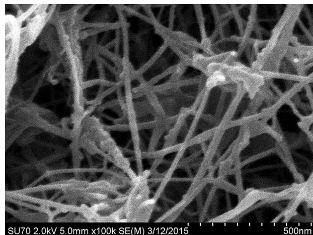
Fig. 1. SEM image of BNNT mat obtained at compaction pressure of 0.47 MPa.
